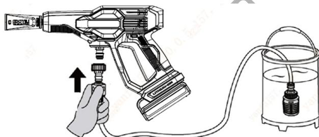
Connect the suction hose (female connector) to the water inlet of the washer and then screw the suction hose (male end) to the open tanks.
