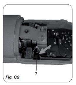
The carbon brushes must be checked regularly. If the carbon brushes are worn, the machine will start to run unevenly.
